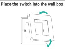
Attach the switch faceplate and cover the screws.
