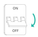
Turn off the power at the circuit breaker for the switch.
